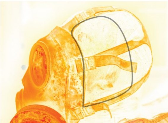
Figure 3 Leakage through a typical gasmask-hood interface.
