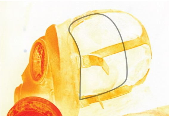
Figure 4 Leakage through the prototype gasmask-hood interface.
