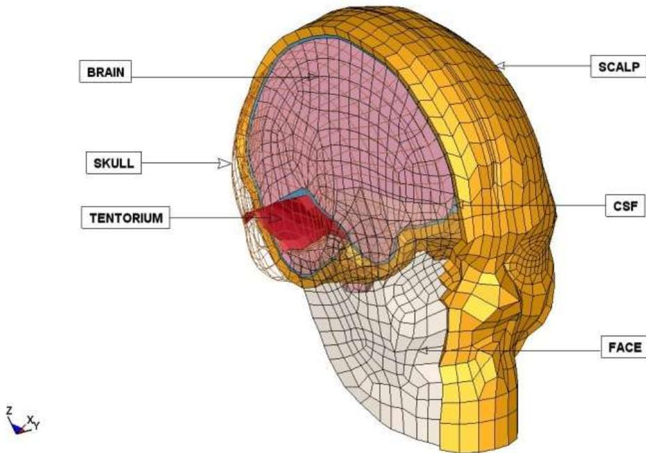
**Fig 1.** Section through the Strasbourg University Finite Element Head Model
