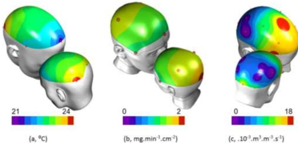
**Fig 1.** Interpolation of air temperature (a) measured at five locations, sweat production (b) measured at four locations and ventilation efficiency (c) measured at 13 locations under a bicycle helmet. Subject tests and manikin head test were performed using the same helmet.
