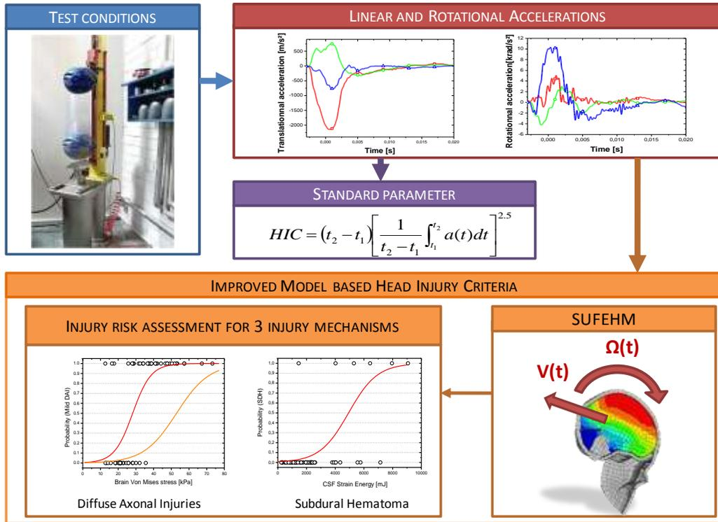
Fig 2. Illustration of the coupled experimental versus virtual helmet test method
