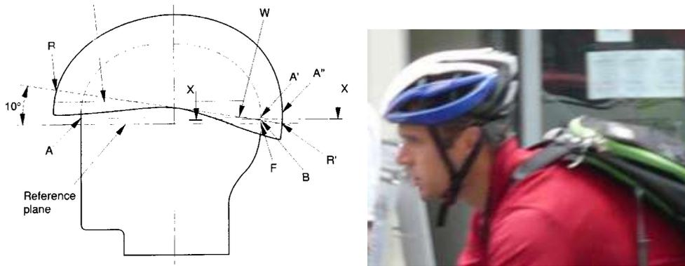
**Fig 1.** a) impact sites in EN 1078 lie above the line  $RR'$ , b) when riding a sport bicycle, the neck is extended to see ahead, and low sites at the rear cannot be hit.
