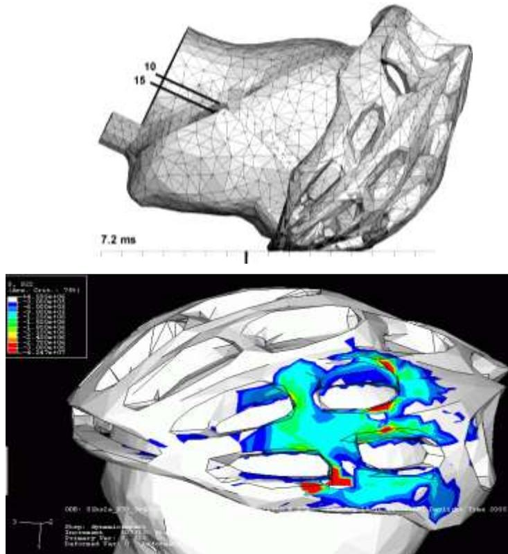
**Fig 3.** FEA predictions the helmet shape in oblique impacts at a) frontal, b) lateral sites
