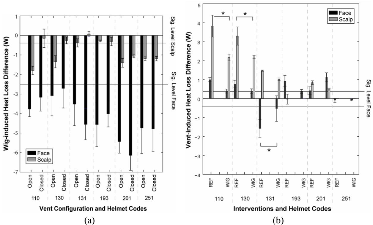
Figure 3: (a) WIG relative to REF, the indicated lines show the significance level ( $p \approx 0.05$ ) as indicated, and (b)  $\Delta C$  of REF and WIG, an asterisk (\*) indicates a significant difference. The error-bars indicate one standard deviation.
