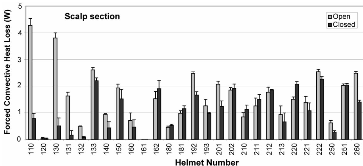
Figure 2: Forced convective heat loss from the scalp section for both open and closed vent configurations as indicated. The error-bars indicate one standard deviation.
