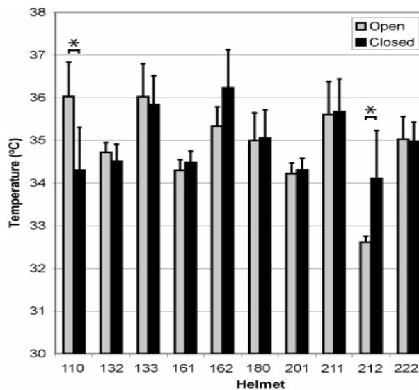
Figure 3: Steady state temperature measured on the top of the scalp (T3) for all motorcycle helmets with ventilation openings closed and open. A \* indicates a significant difference ( $p < 0.05$ ) upon changing the ventilation openings.
