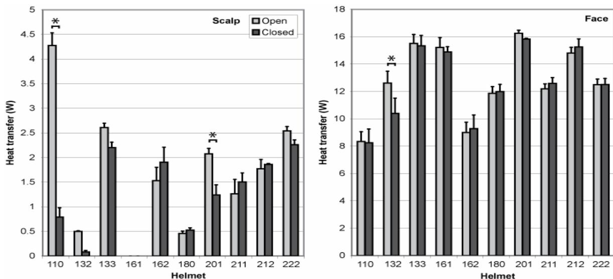
Figure 2: Steady state heat transfer for the scalp and face sections as indicated, measured for all motorcycle helmets with ventilation openings closed and open. A \* indicates a significant difference ( $p < 0.05$ ) upon changing the ventilation openings.
