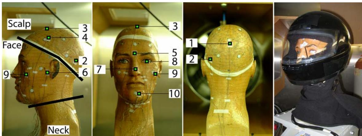
Figure 1: Thermocouple location on the thermal manikin headform. The locations of the 10 thermocouples are indicated with squares and corresponding numbers. The three sections are also indicated. In the right most picture the headform is shown with a motorcycle helmet.
